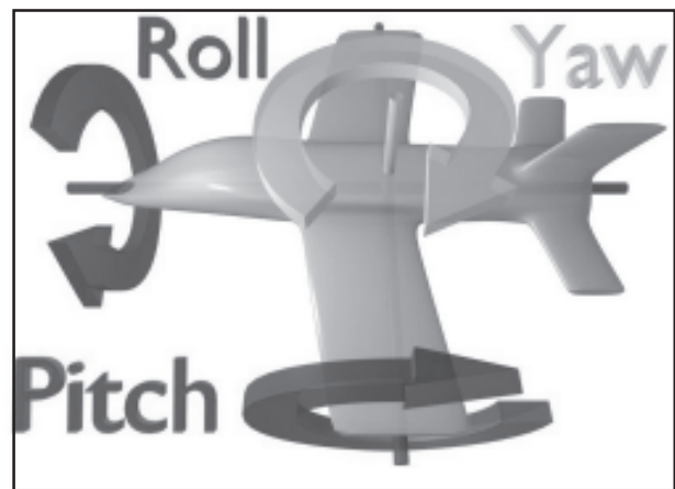
Fig.1 - Description of pitch, roll and yaw in INS (en.wikipedia.com)
